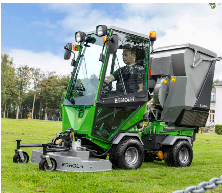
Rotary/mulch mower 1000 with grass collector
